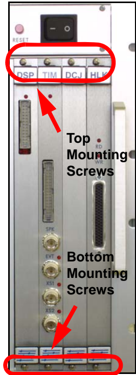
Figure 2 MAP Board Mounting Screw Locations
