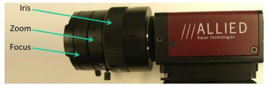
Use the physical settings on the camera lens to obtain the best possible image. Do this before configuring any camera settings in the CinePlex software.
